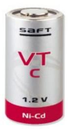
The VT C cell is designed to accept a permanent charge (C/2O) for a minimum of 4 years in high temperature environnements (up to +  $55^{\circ}$ C) such as security lighting installations.
