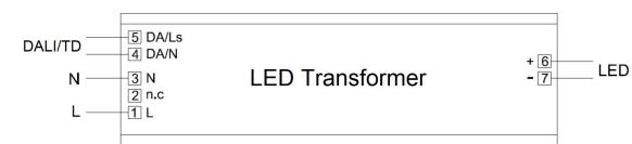
For independent application: minimum wire cross section = 0.75 mm<sup>2</sup> / 18AWG for output current > 2A
